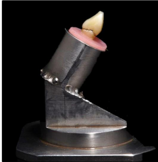
Figure 1. Specimen in the load device. Cyclic isometric loading was applied to the incisal edge at an angle of 30°.
